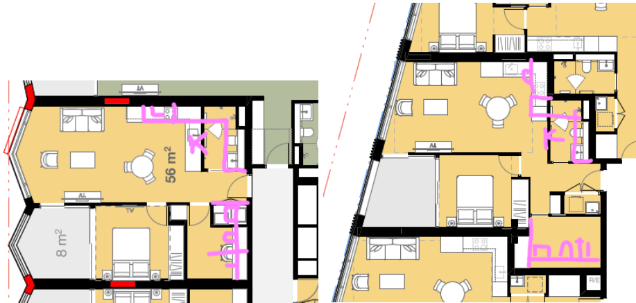
Figure 17 and 18: Sketch of re-design relocating bathrooms to studies and increasing living area
