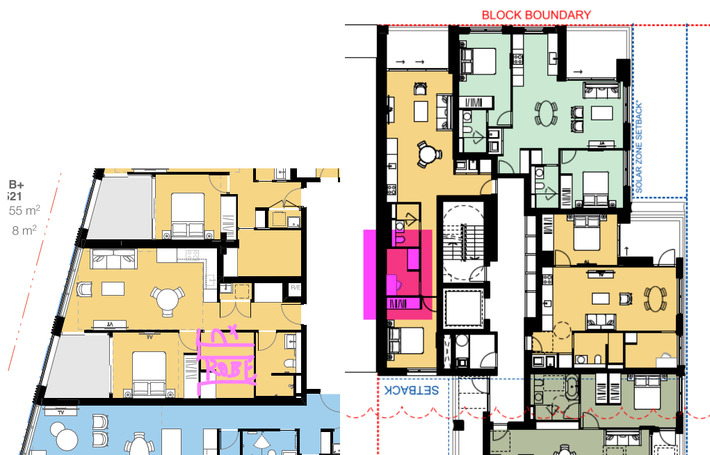
Figure 19 and 20: Sketch of re-design replacing studies with walk-in robes
